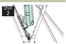
Attach the battery and let its cable through the bottom of the bottle cage.
