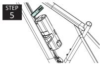
Tie the rubber strap over the battery and bottle Adjust the rubber strap to ensure the battery is cage back.
